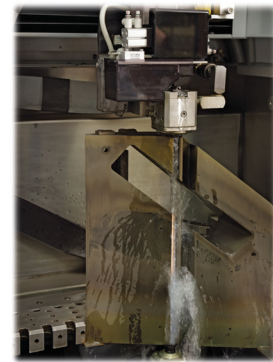
Wire EDM capability to 13.5" thick
